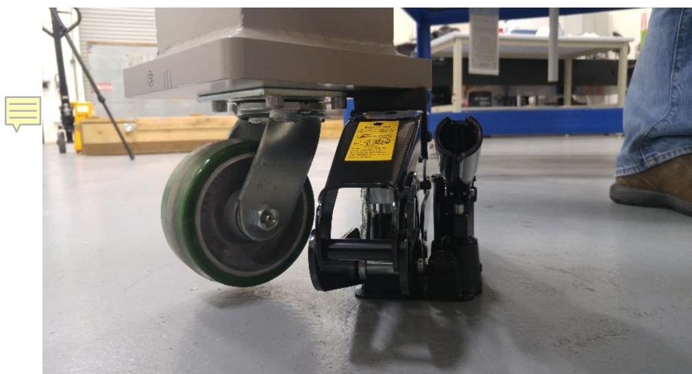
Figure 28 – Level the integration table using lifting jacks under the legs as necessary.
