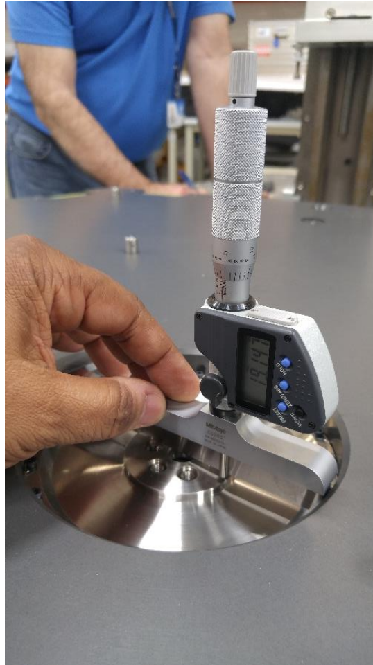
Figure 8 – Measure the vertical distance from the top of the parallel bar to the top of the central boss of the central diaphragm.
