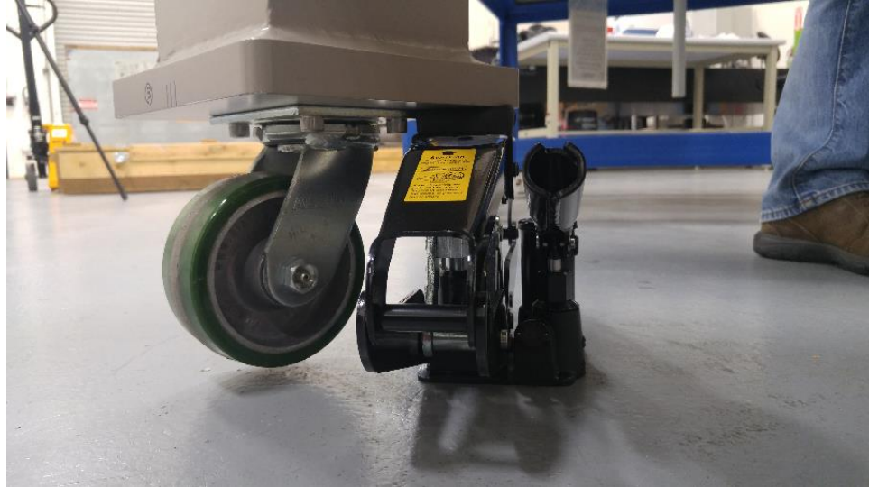
Figure 39 – Level the integration table using lifting jacks under the legs as necessary.
