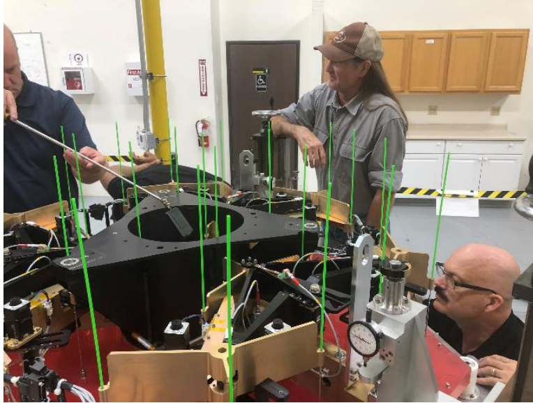
Figure 49 – Lowering the SSA towards the segment for final integration.
