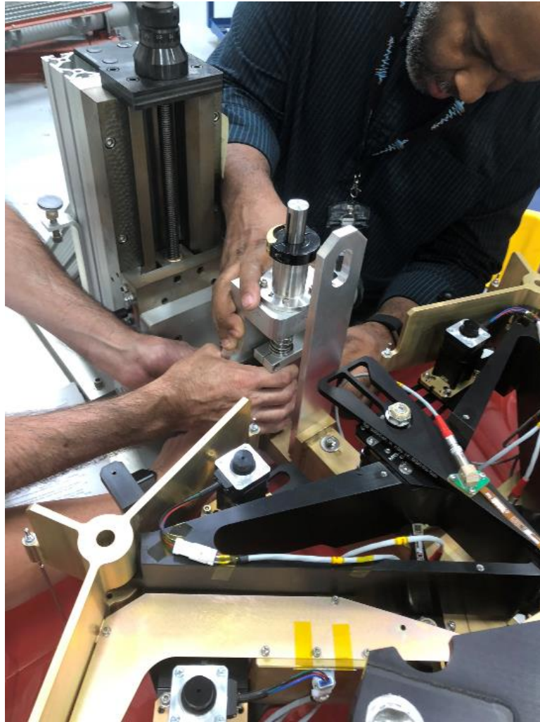
Figure 58 – Removing the collar clamp to release the Delrin balls.
