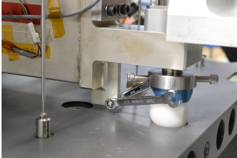
Figure 56 – Torquing the tangential restraint arm fasteners.
