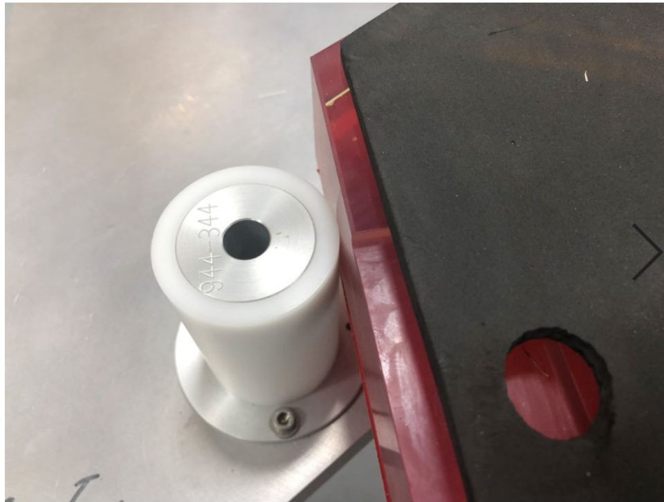
Figure 6 – Place the segment on the integration table so that it is touching the three fixed circular pads as shown.
