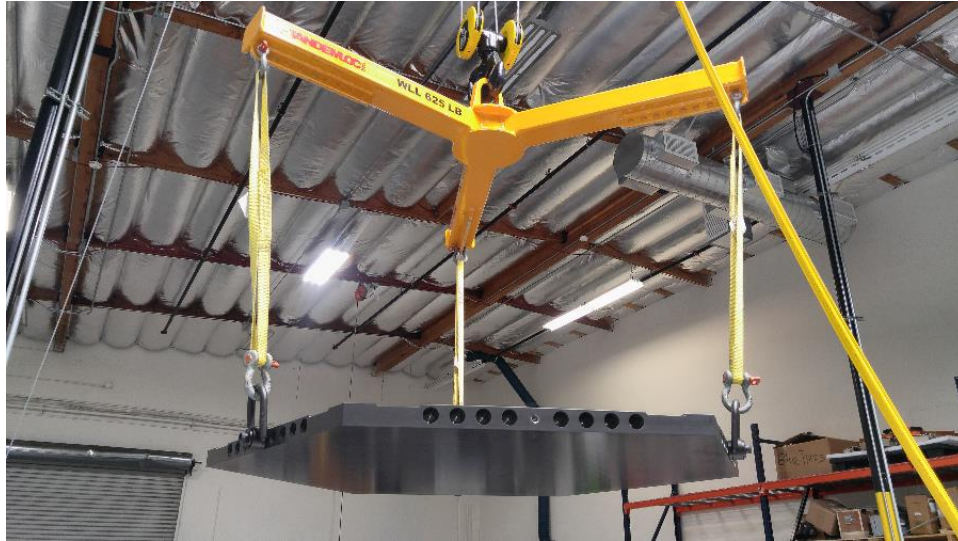
Figure 4 – Craning an aluminum dummy segment. The S2 surface is uppermost.
