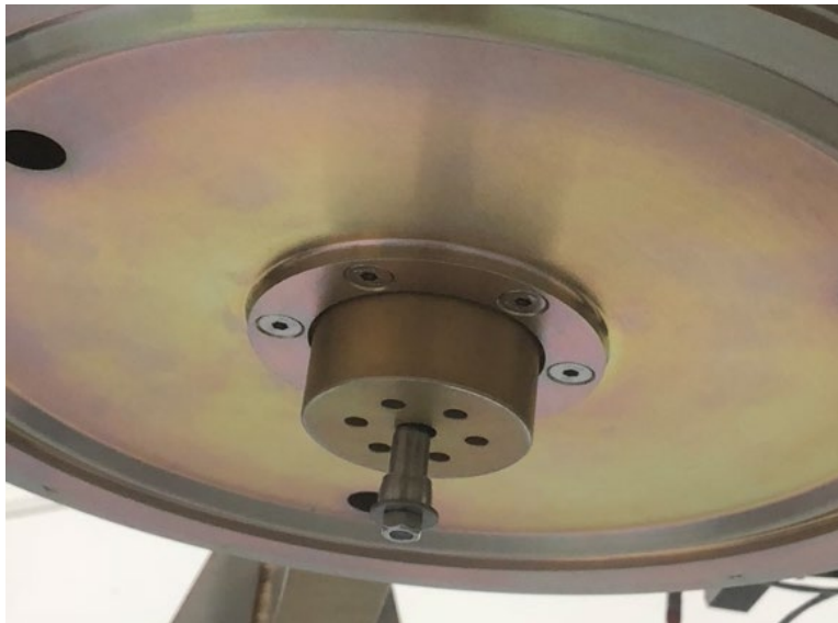
Figure 26 – The center boss as it is pressed into the moving frame hub.
