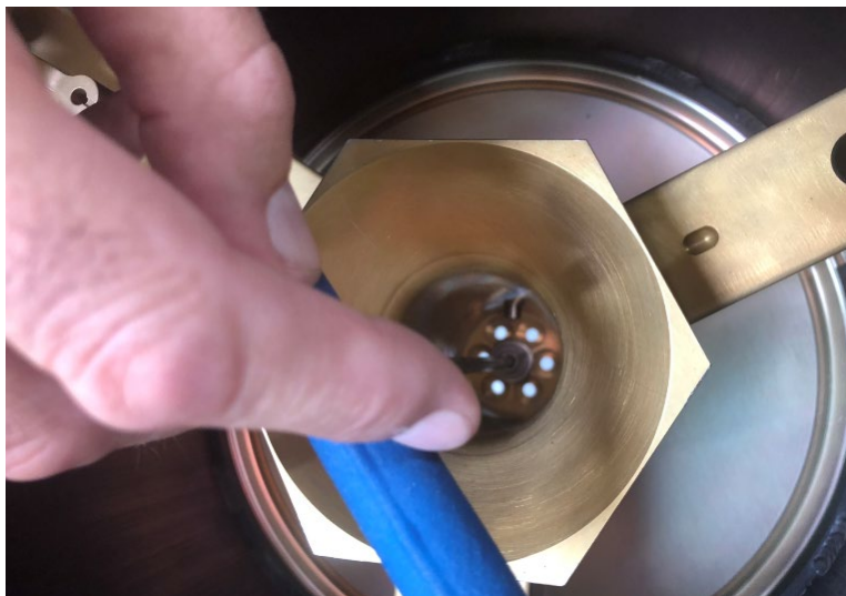
Figure 27 – The T-handle Allen wrench from the top view, while the center boss is pressed into the hub.
