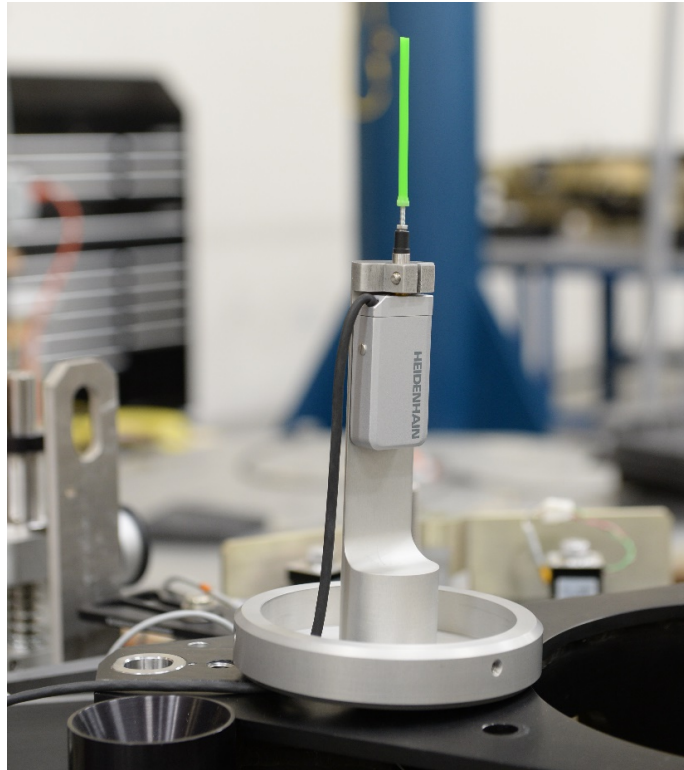
Figure 14 – The LVDT in its holder, with a 75mm green extension straw attached.
