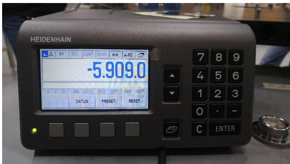
Figure 15 – The Heidenhain ND 287 Display Unit used to read the LVDT.
