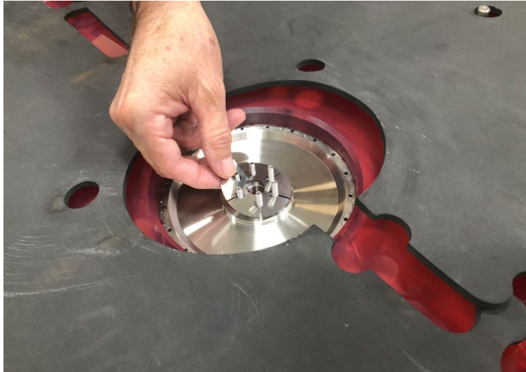
Figure 32 – The calculated diaphragm shim-stack placement.
