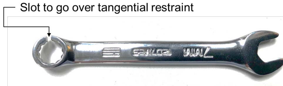
Figure 55 – Custom 7 mm wrench for use with the tangential restraint fasteners.
