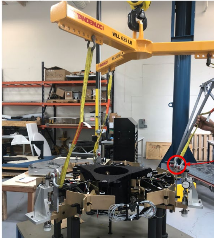
Figure 13 – Lifting equipment in place, ready to lift the SSA.
