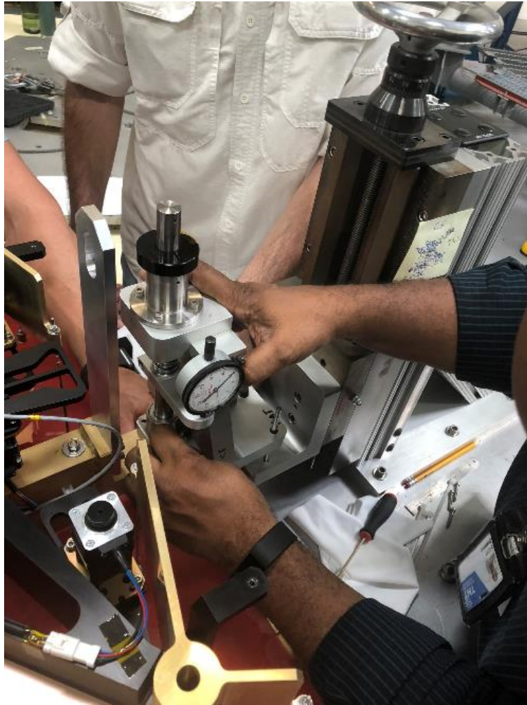
Figure 59 – Unbolting the dial indicator brackets.
