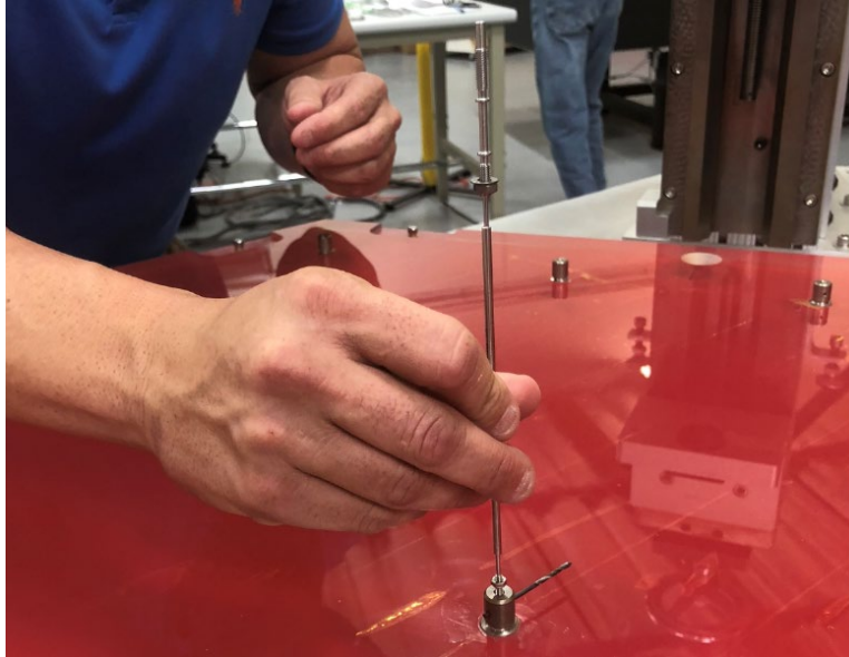
Figure 33 – The installation of the MRF with a drill bit and the lower and middle nut-washer sets in place.
