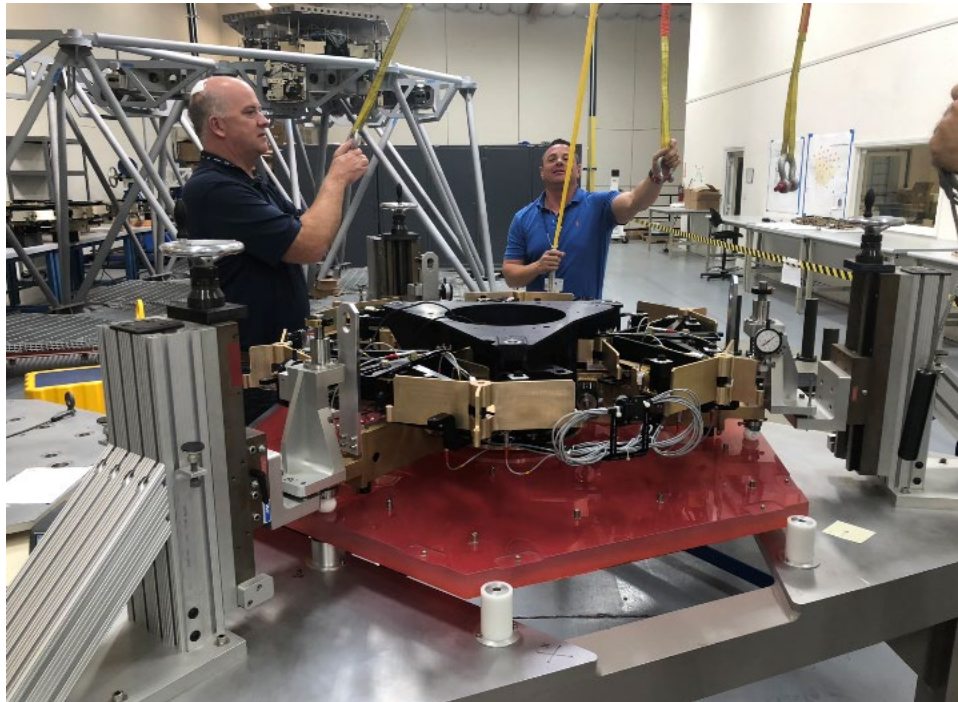
Figure 22 – Lowering the SSA towards the segment for shim measurement.
