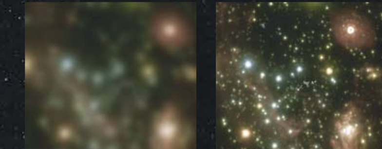
Keck AO-image of Galactic Center (right) contrasted with simulated non-AO image (left).
